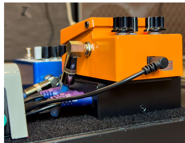
Pro Tip: Photo showing an XP5 being used as a pedal riser on a pedalboard.
