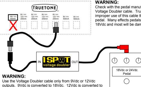
24Vdc. Do not use with input voltage greater than 12Vdc.
